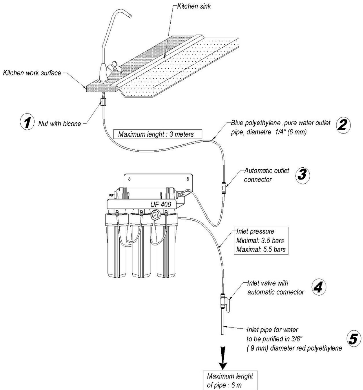
1. The nut with bicone must be tightened on to the tap gently. As a rule, it is sufficient to tighten hard by hand on to the tap stem to provide sealing. Should this not be sufficient, it may be tightened gently using a tool. In all cases, **stop tightening once it is sealed.**
