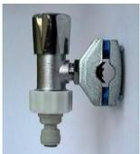
DIR - 01: this self-tapping valve can connect directly to a copper water supply pipe of 10, 12, 14 or 16 mm diameter without any special tools other than a simple screwdriver. It is then fitted with the RAC - 01 automatic connector for direct connection of the purifier.
